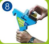
Squeeze lever and keep closed. The FlexiTag is in cutting position. Slide to the loader/cutter fully back. Tag is now cut.
