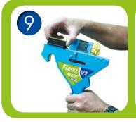
Firmly slide loader to forward locked position. The FlexiTag is now loaded.
