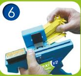
Slide the rolled FlexiTags into the drum.
