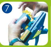
Depress the clamp firmly. Slide tags out until location lugs are between first and second tag.
