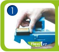
Ensure loader/cutter is in locked position (at front of applicator).
